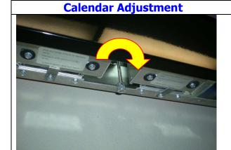
The calendar knob turns **clockwise only** and should **NOT** be pulled down.
