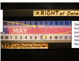
Since Paris is to the left of the dateline, the bottom row is used. Most of May 7<sup>th</sup> has passed from the perspective of the international dateline, so the black indicator line is close to the line separating the 7<sup>th</sup> and the 8<sup>th</sup>..
