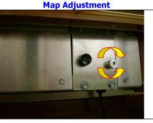
The map knob must be pulled down to disengage it from the motors. It can be turned either direction.
