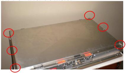
3) Removing the front panel: There are 4 nuts to be removed from the bottom and 3 screws to be removed from the top.
