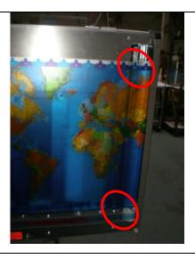
The compression springs will be located as highlighted in the photo, behind the map and between the frame and the take-up roller. Oftentimes they can be reached by "fishing" them with a screwdriver or possibly just with fingers.
