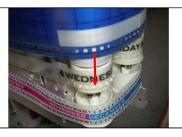
Gently pull the map over the day of week band, aligning the perforations as best as possible. Slide the map perforations over the roller sprocket
