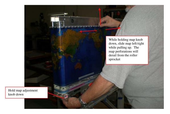
Once the map is off the sprocket teeth, jostle the map side to side while pulling up gently, making sure it doesn't catch any brackets or screws on the way up
