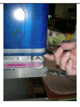
Ensure map is <u>NOT</u> riding in the sprocket of the rear roller by holding the map away with your finger.
