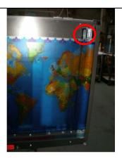
Insert the top spring first, just above the map. Ensure it is in far enough to allow for full compression of the roller plate.
